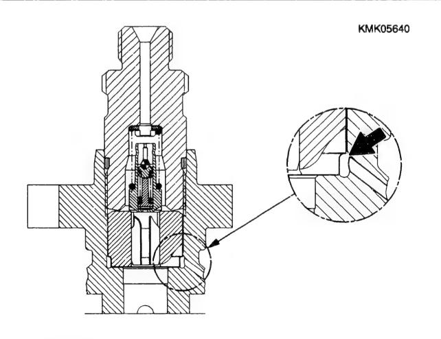
Valve cone and valve holder have a defined sealing seat, the sealing surfaces of which are specially machined. If the valve cone is inadvertently inserted into the opposite side of the valve-holder bore (shoulder then faces upwards), leakage will subsequently result and become apparent in the form of:
